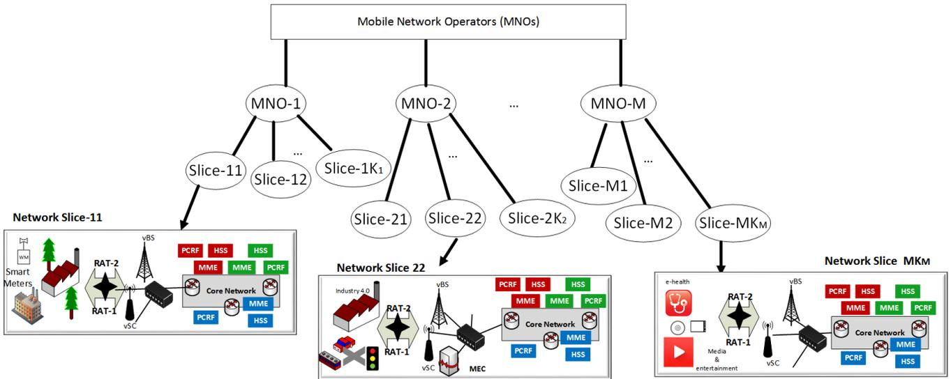
Fig. 1: Network slicing for multiple MNOs having different services and applications.
