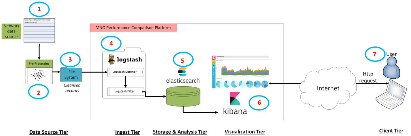
Fig. 2: Demonstration Setup
