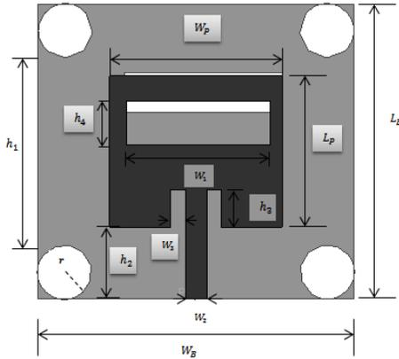
Fig. 4: Top and Bottom View of the Proposed Dual Band Antenna
