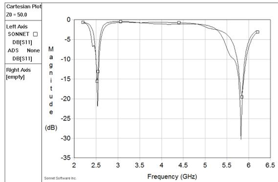
Fig. 5: Input Reflection Coefficients (S11) of Proposed Antenna
