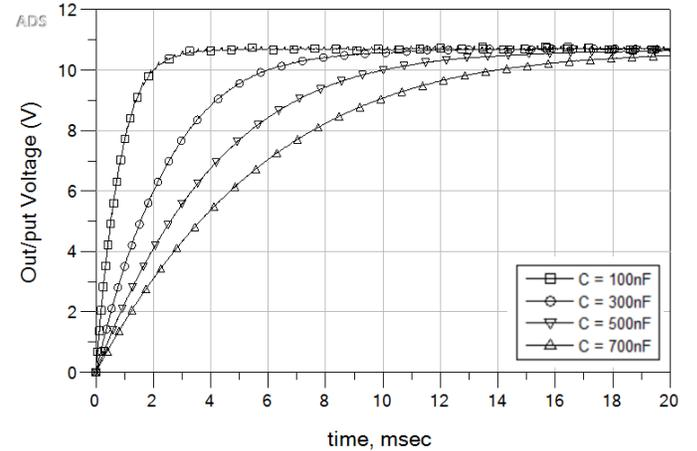
Fig. 9: Output Voltage versus Time at load=10k on Different Storing Capacitors (nF)
