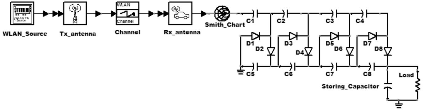
Fig. 3: System Architecture of Proposed System
