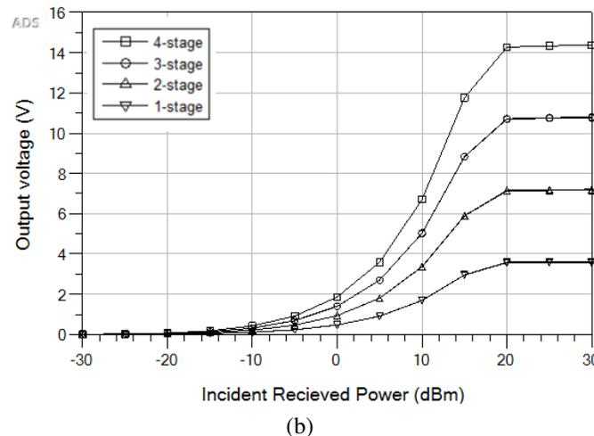
Fig. 8: (a) Output Voltage versus  $P_r$  (-30dBm to 5dBm) (b) Output Voltage versus  $P_r$  (-30 dBm to 30 dBm) at load=10 kΩ
