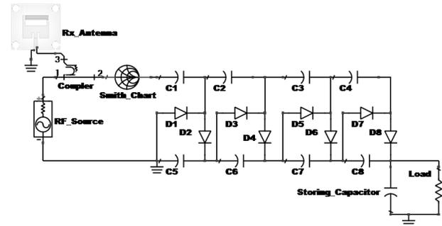
Fig. 2: Schematic Diagram of 4-Stage WLAN Energy Harvesting System
