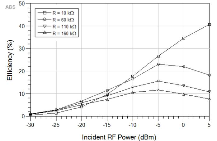
Fig. 10: Efficiency (%) versus Input RF Power (dBm) at Different Loads (kΩ)
