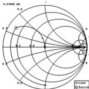
Fig. 6: Impedance Matching using Smith Chart on ADS Agilent
