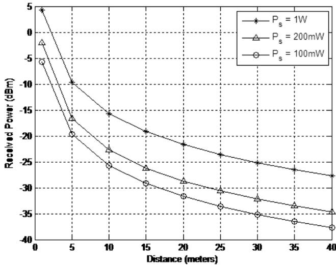
Fig. 7: Received Power ( $P_r$ ) vs. Distance at different Source Power ( $P_s$ )
