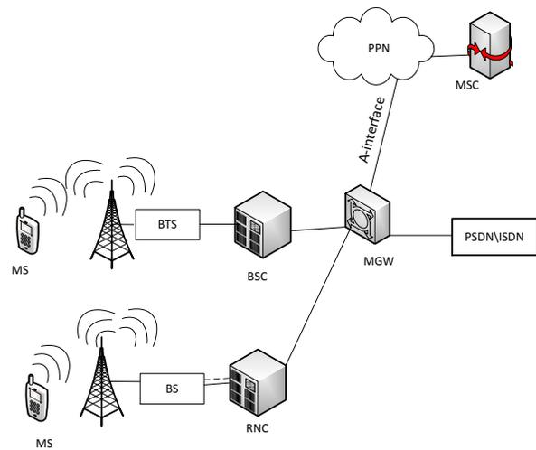
Fig. 1. Cellular network architecture and mirroring of A-interface in the network
