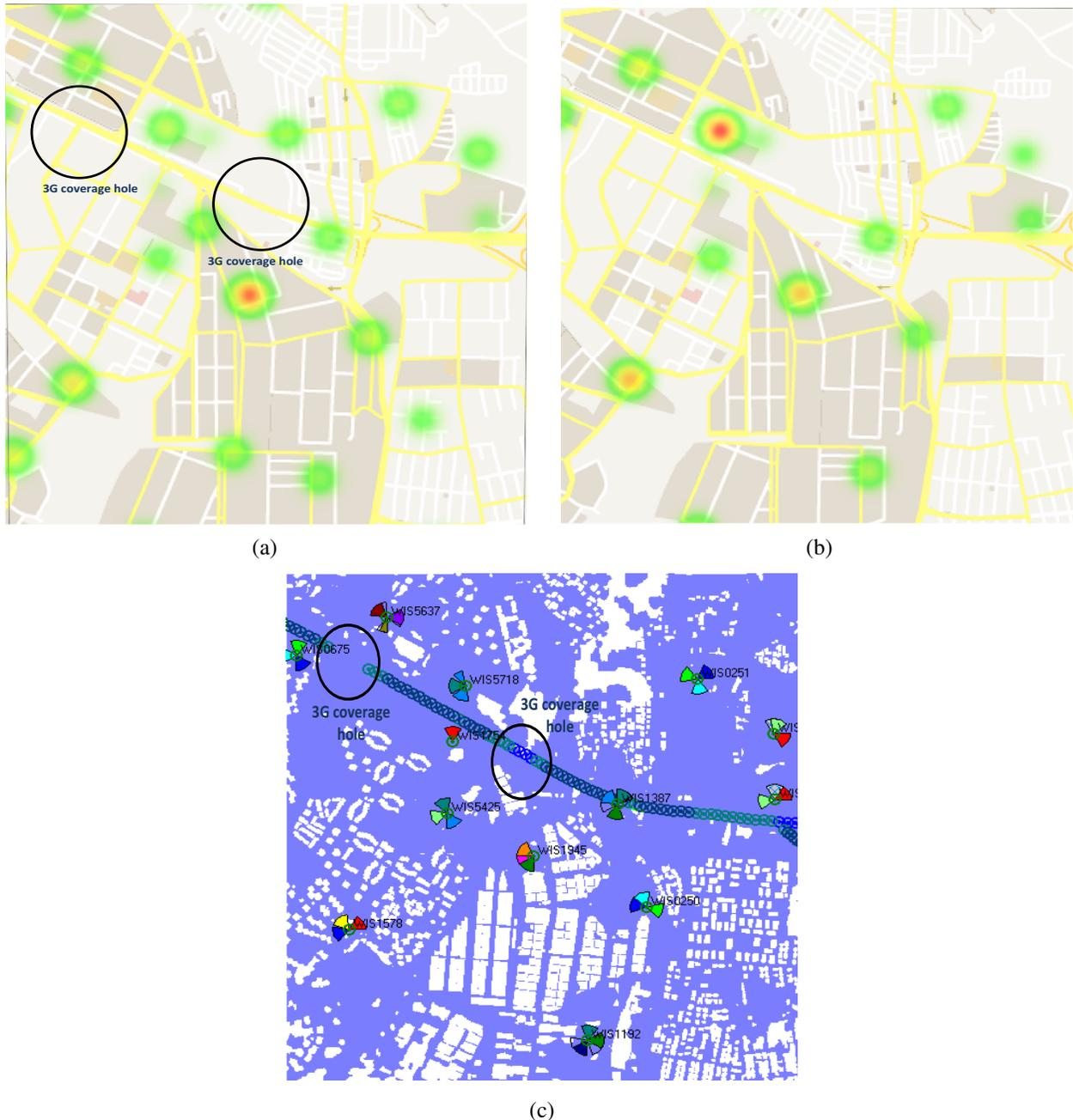
Fig. 3. (a) Google map illustration for 3G coverage hole identification using the proposed platform. (b) Base station IRAT HO KPI heatmap. (c) Drive test results on the same area.
