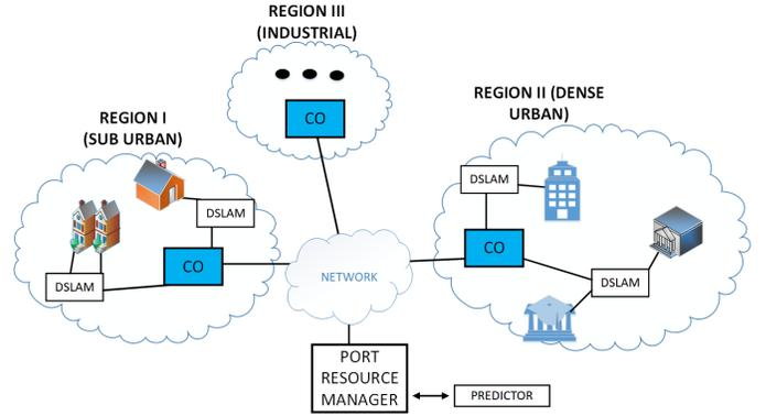
Fig. 1: System architecture illustrating DSLAM, CO, port resource manager and proposed predictor.
