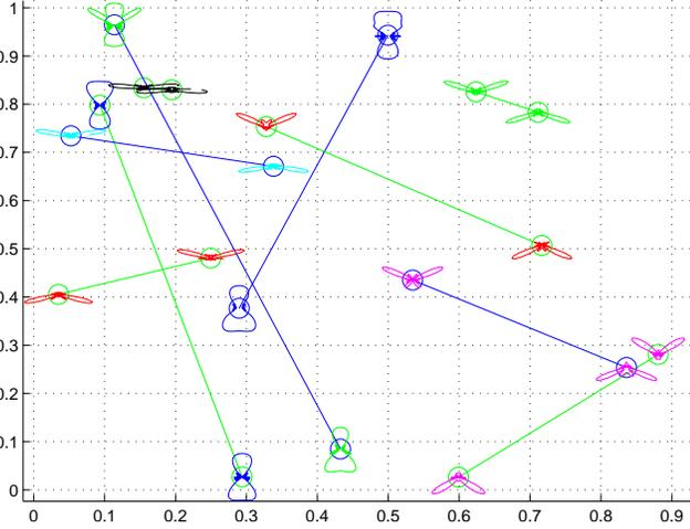
Fig. 2. Considered scenario and node positions with beamform patterns of 20 nodes which are distributed in a 1x1 square meter area.
